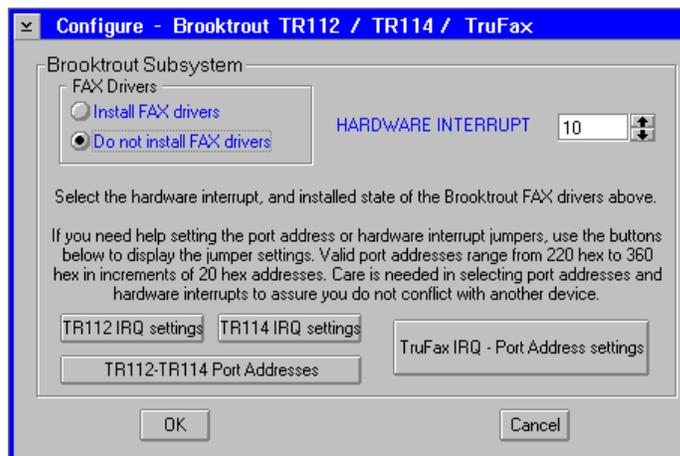
3. The FAX Drivers box indicates the current state of the Brooktrout board drivers. If the drivers are not installed, select the Install FAX drivers option to load the drivers upon bootup. If you remove the Brooktrout boards later, you can select the Do not install FAX drivers option to make sure the drivers are not loaded.
